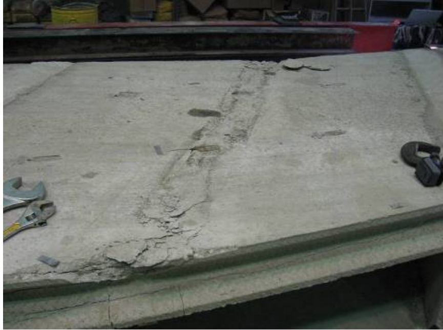
a) deck panel after loading
