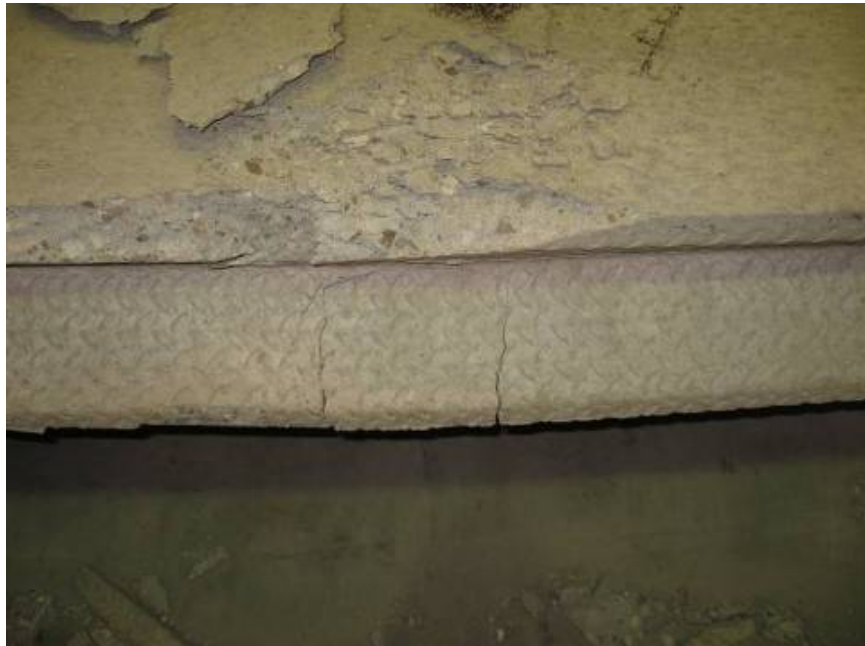
a) deck panel after loading
