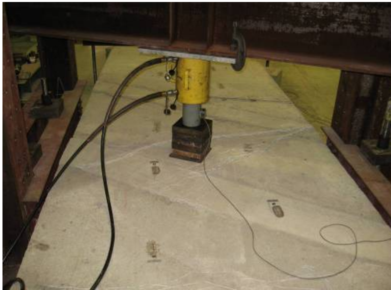
b) test setup for closure joint ultimate load test
